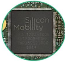
HVIC 2.1 board with OLEA® FPCU T222 mounted on PM100 inverter
