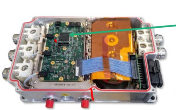
HVIC 2.1 board with OLEA® FPCU T222 mounted on PM100 inverter
